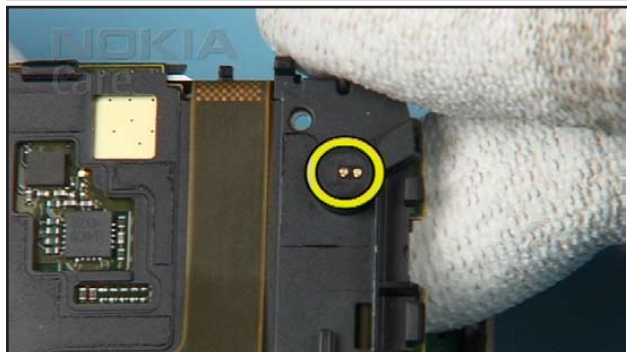
16. Remove the MICROPHONE and discard the UI MODULE.
