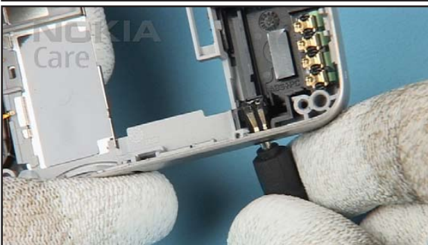
31. Remove the DC-JACK with the DC-Plug.
