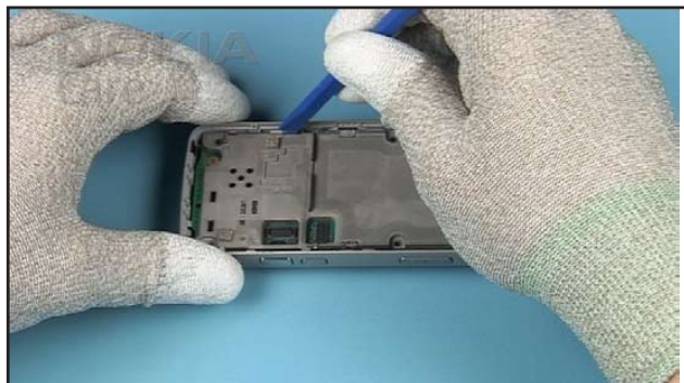
22. Unlock the MAIN FRAME ASSY starting at the shown side.
