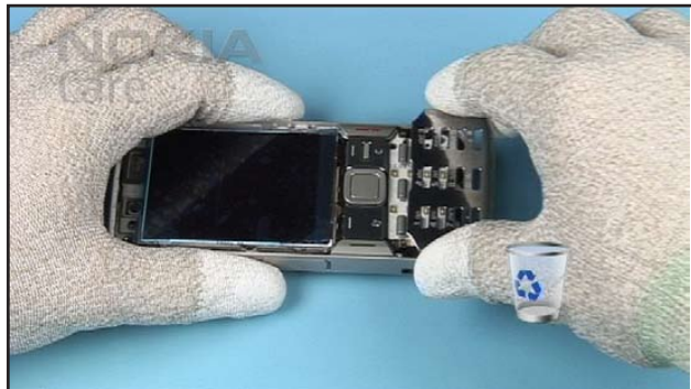
10. Remove the KEYMAT COVER and discard it.
