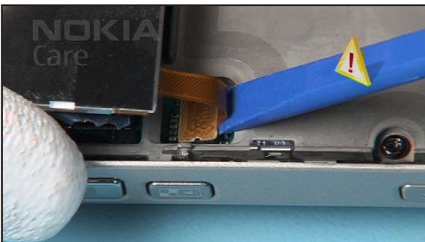
19. Gently open the LCD connector.
