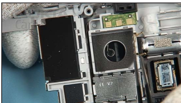
37. Carefully remove the CAMERA GROUNDING SPRINGS.
