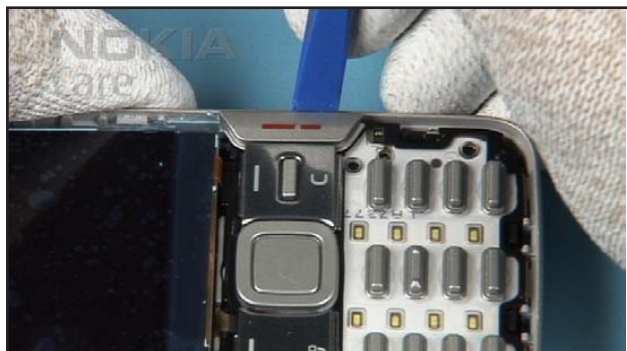
12. Unlock both side snaps. Avoid damaging of the B-COVER.
