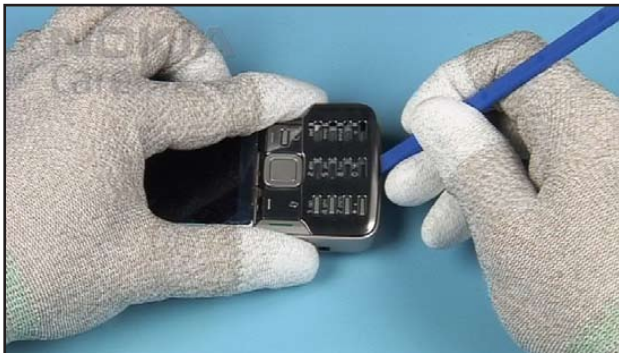
9. Unlock all clips of the KEYMAT COVER.
